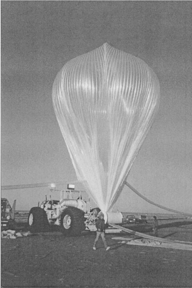
Fig. 1 Spool configuration of large scientific balloon.
